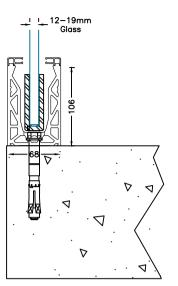
Concrete 4000 PSI Minimum Steel 12mm Thick Minimum
